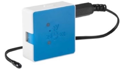
Figure 4: Pocket Lab Weather sensor with temperature probe
